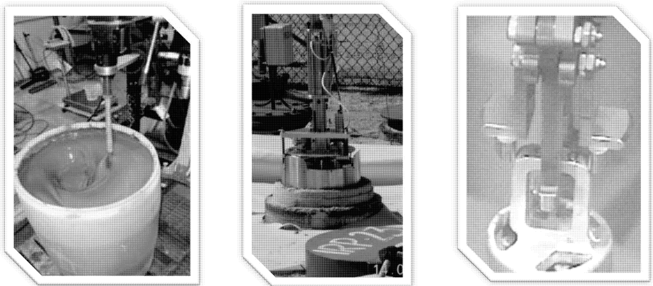
Figure 8 Full scale testing of Cement formulations to support liquid/sludge inventories (left). Cemented Molybdenum-99 Waste Retrieval Tool (middle) NRU Fuel Cap Grapple (right)
